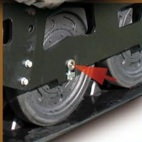
Grease lubricated wheel axles for enhanced longevity.
