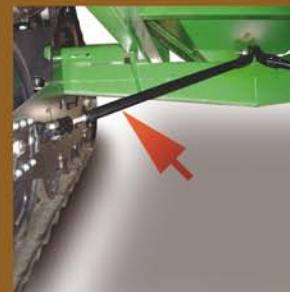
Simple torsion bar reinforcement adapts to most grain carts.
