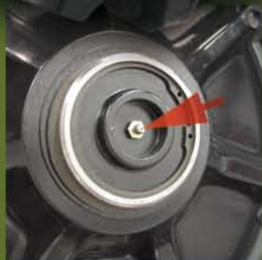
Grease lubricated wheel axles for enhanced longevity.
