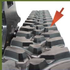
Rubber track profile designed for increased flotation and high load applications.
