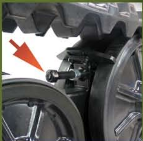
Simple track tensioning system designed for easy access.
